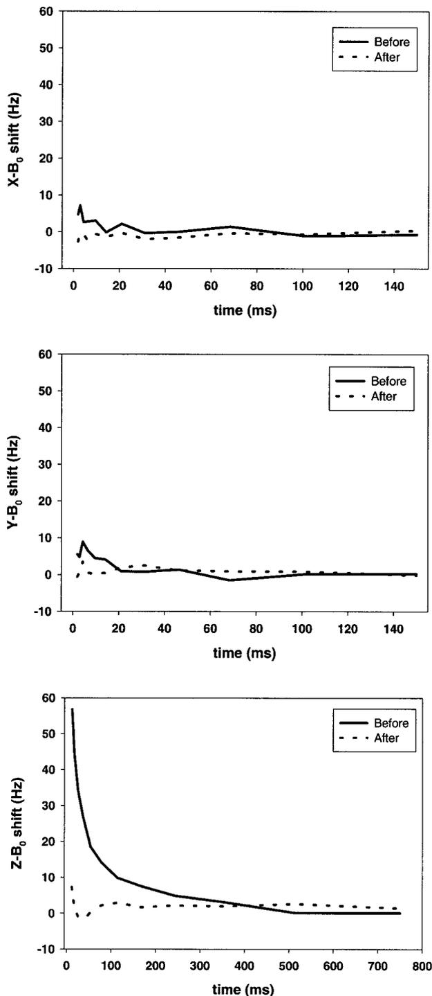
FIG. 5. Plots of  $B_0$  shift generated by  $x$ ,  $y$ , and  $z$  gradients of 30 mT/m strength and 20 ms duration with no  $B_0$  compensation (solid line), and with calculated  $B_0$  compensation (dashed line).
