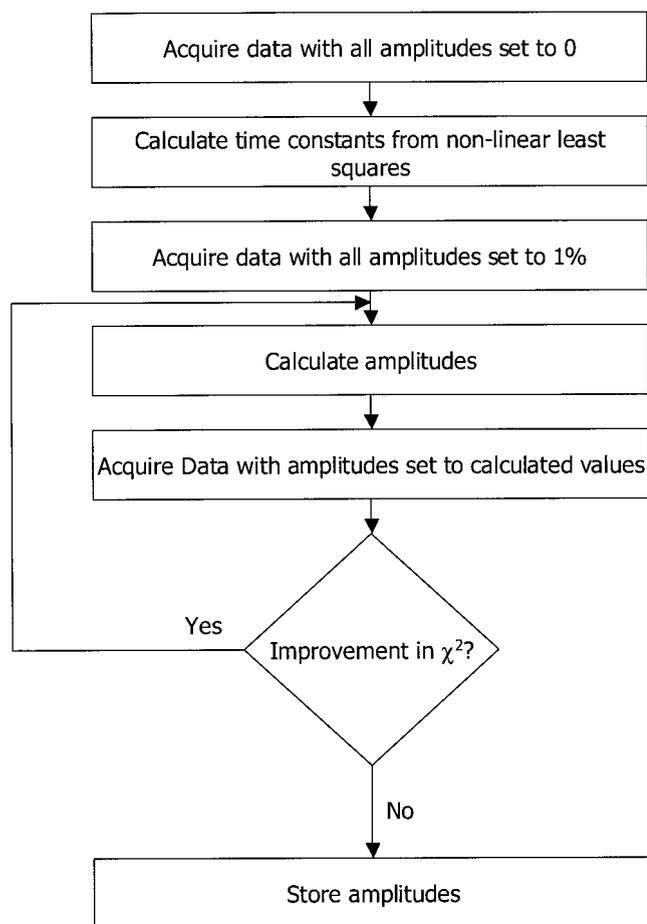
FIG. 3. Flowchart of the procedure used to automatically determine the optimal time constants and amplitudes of the preemphasis unit for a given gradient direction.
