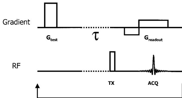
FIG. 1. Diagram of the pulse sequence used to estimate gradient eddy currents.  $\tau$  is the variable delay.
