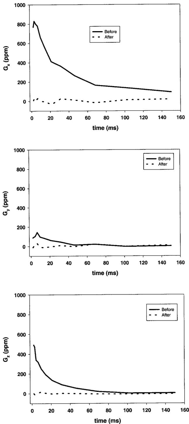
FIG. 4. Eddy currents generated by  $x$ ,  $y$ , and  $z$  gradients of 30 mT/m strength and 20 ms duration with no preemphasis compensation (solid line), and with calculated preemphasis compensation (dashed line).
