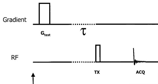
FIG. 2. Diagram of the pulse sequence used to estimate  $B_0$  eddy currents.  $\tau$  is the variable delay.
